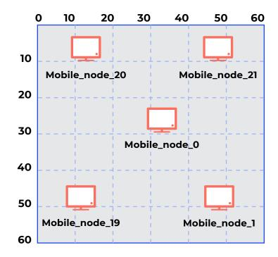
Here we show a simulation in OPNET with a network of five nodes, all with 11 Mbps data rate, but one of them changes its rate with time as a control node.
